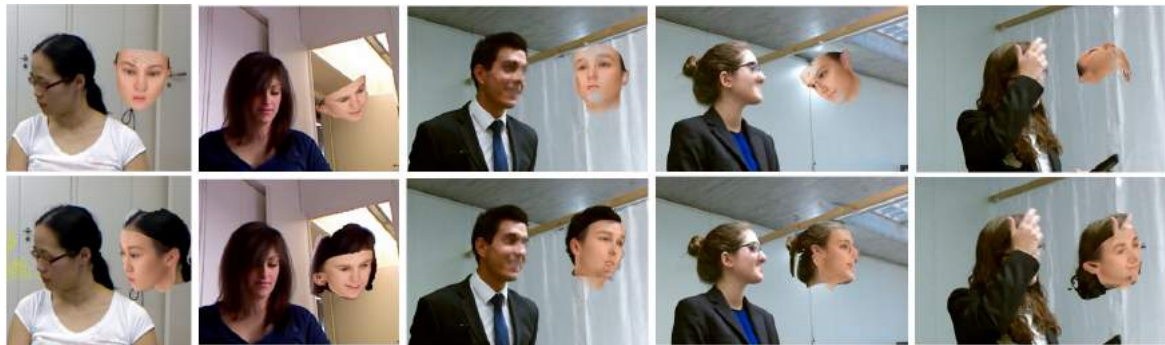
Figure 17: Results of head pose estimation using only the 3DMM (top) and augmented model (bottom).
