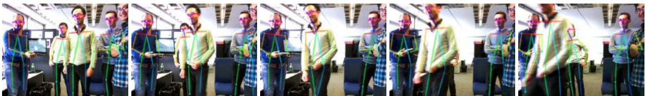
Figure 11: Output of the system of video recorded from Pepper. The images show the articulated poses overlaid on the image containing multiple people.
