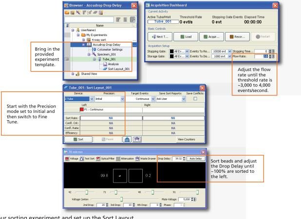
Open your sorting experiment and set up the Sort Layout.
