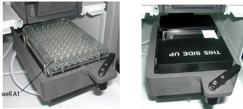
Figure 5-4 ACDU stage set up with plate (left) and slide (right)
