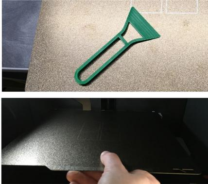
B – Use the plastic scrapers to remove any remaining material from the build plate. Carefully guide the build plate back on to the platen, ensuring it is keyed in and lay flat.
