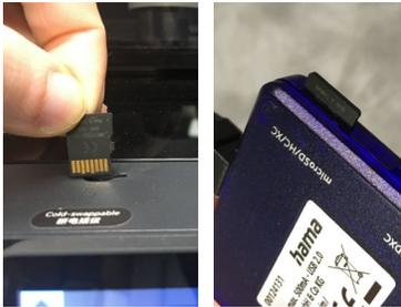
B – Remove the MicroSD card from the front of the machine with a gentle press to eject it. Carefully put the card into one of the card readers drop-down insert the card reader’s USB into your laptop.
