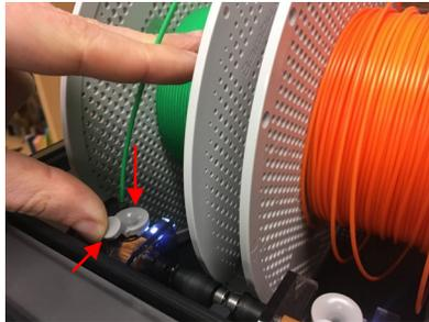
B – If it is necessary to switch spools between bays, gently push the tab of the feeder towards the spools, then feed the material in carefully until the machine pulls the material automatically.
