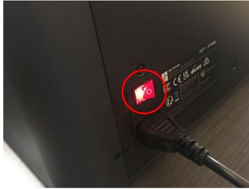
**A – The printer’s MicroSD cards are cold swappable, meaning the machine must be switched off when the card is removed and inserted, to avoid file corruption. The switch to turn the printer off is on the back of the machine, right side when facing. Press the buttons on the LCD screen if you are unsure if the printer is on/off.**
