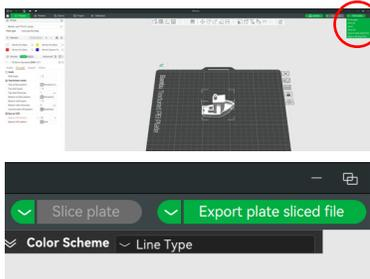
C – Once your model has been sliced and the project file saved, the G-code can be exported to the MicroSD. Select “Export Plate Sliced File” from the drop-down menu on the top right side of the screen then confirm. From here the G-code can be saved. Give your file a recognisable name. Safely eject the MicroSD.
