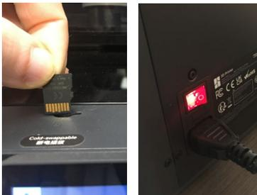
D – Insert the MicroSD back into the switched off machine. Following this, the machine can be switched on.
