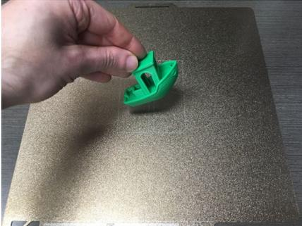
A – When the print is complete, carefully remove the build plate from the printer. Separate the model from the plate by bending the plate, or carefully use a plastic scraper to assist.
