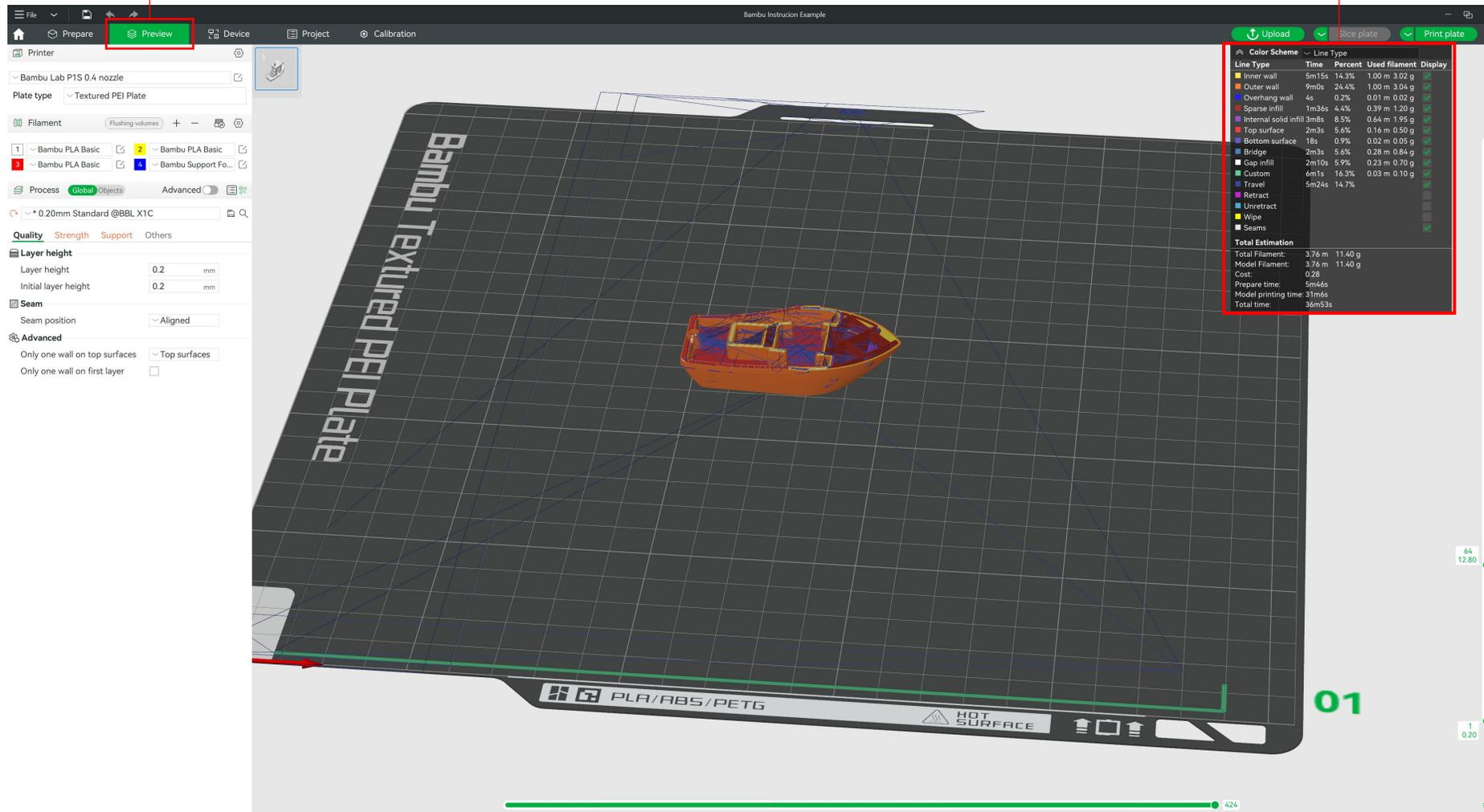
The screenshot shows the Bambu Studio software interface. The main window displays a 3D model of a boat on a printing bed. The left sidebar contains printer settings, including filament type (Bambu PLA Basic), process (0.20mm Standard @BBL X1C), and quality settings. The top menu bar includes 'Prepare', 'Preview', 'Device', 'Project', and 'Calibration'. The right sidebar features a 'Line Type' table and a vertical slider for layer-by-layer slicing.
