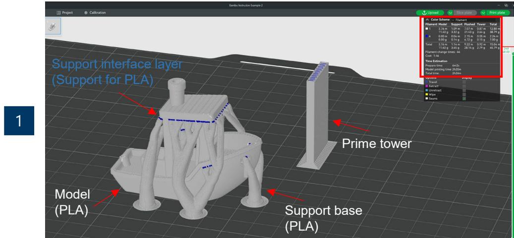
Note: Two filaments being used, and time estimation and material used. More changes = more time & material waste
