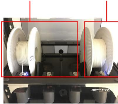
A – The filament spool bays should be laid out in the configuration shown. Check whether the spools are empty or near empty. There are markers on the side of the spools indicating the number of grams of material remaining. If there doesn't appear to be enough material for your model, use another printer.
