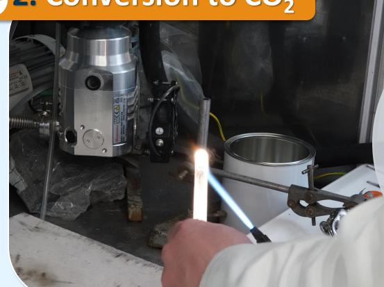
Samples are converted to CO<sub>2</sub> either by combustion in sealed quartz tube (organic materials) or acid hydrolysis (carbonates).
