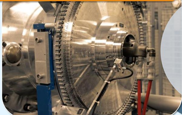
The graphite targets are analysed by accelerator mass spectrometry for radiocarbon measurement / dating.
