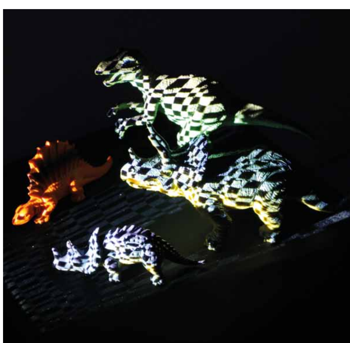
The process of "structured illumination": the objects are illuminated with a rapid series of patterns that resemble crossword puzzles, generated by a digital light projector
